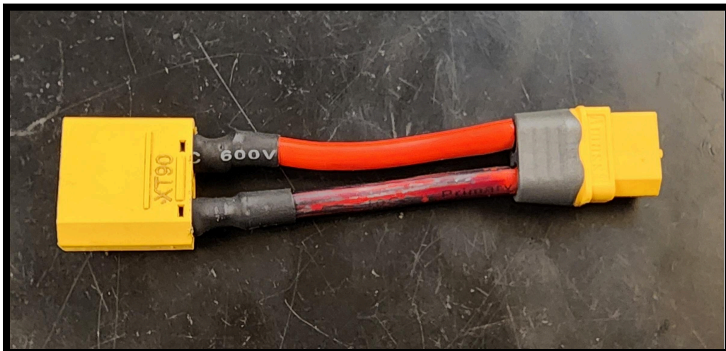
Figure 6: Adapter to Connect VESC and Battery Pack
