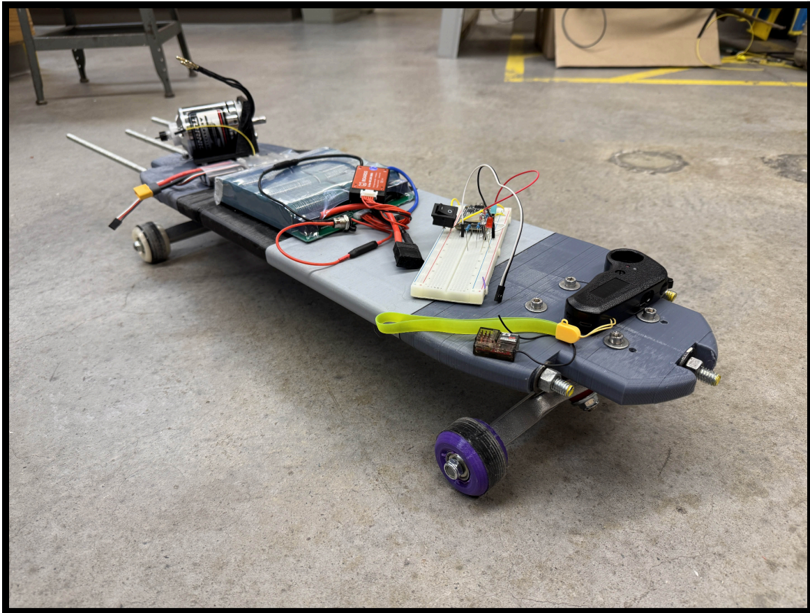
Figure 1: The Assembled Board With Electronics on Top
